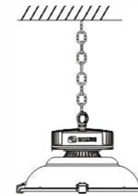
Hanging chain installation
