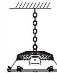
Hanging chain installation
